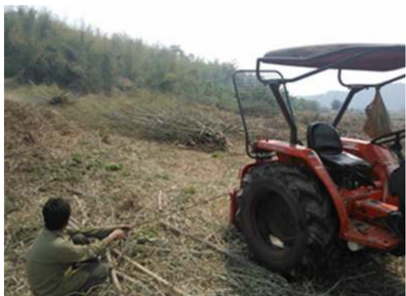
Figure 17. Extraction of bamboo using Jewel 3 to winch with a Kubota 35 HP farm tractor
