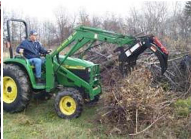
Figure 7. Front grapple loader ( www.worksaver.com/product/compactgrapple.html ).
