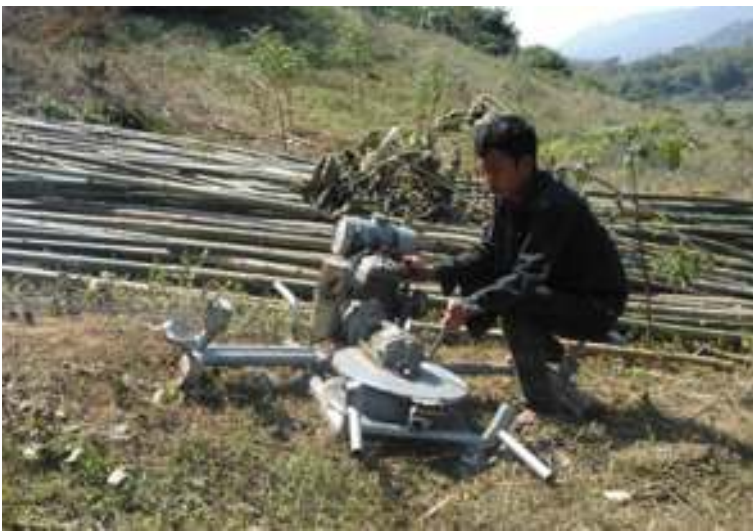
Figure 6. Werner Ziehmax vineyard sledge winch used in bamboo extraction, Bokeo province, northern Lao PDR.
