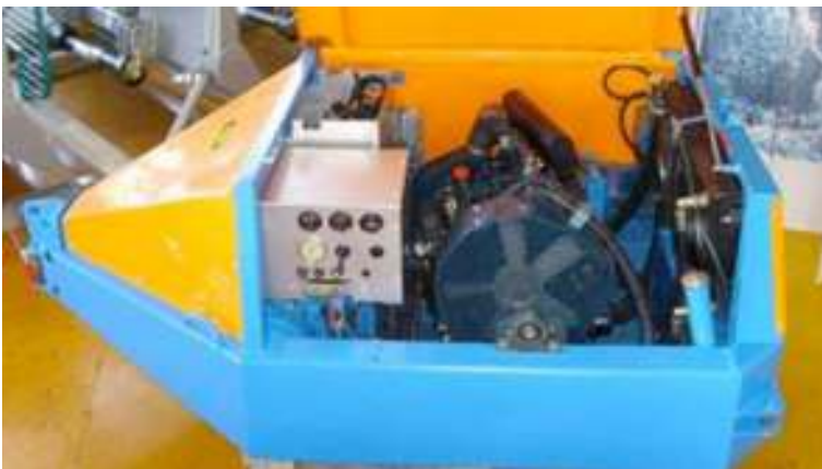
Figure 7. Interior of the Waldrapp 32-hp motor sled winch
