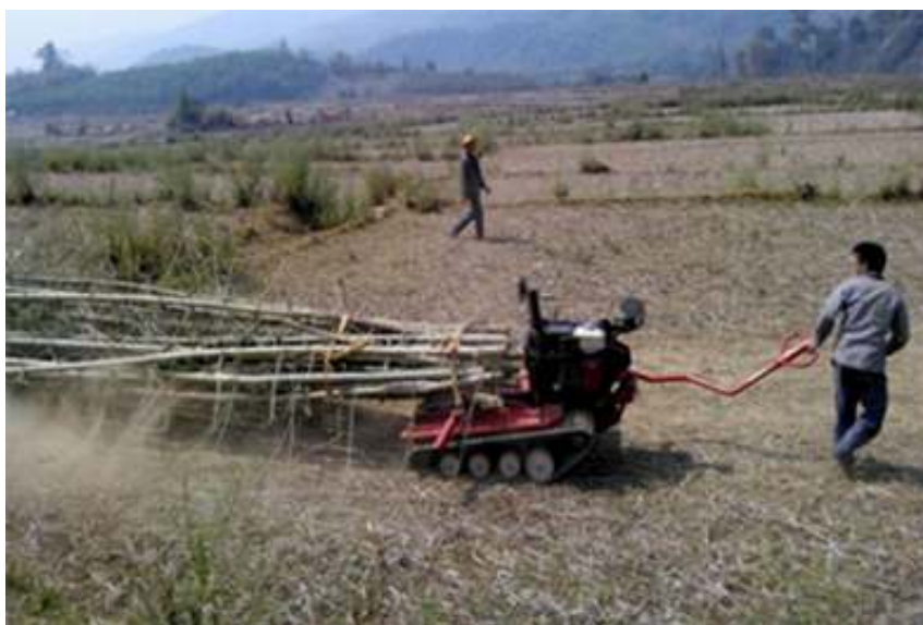
Figure 14. Forwarding bamboo culms with branches using an Iron Horse
