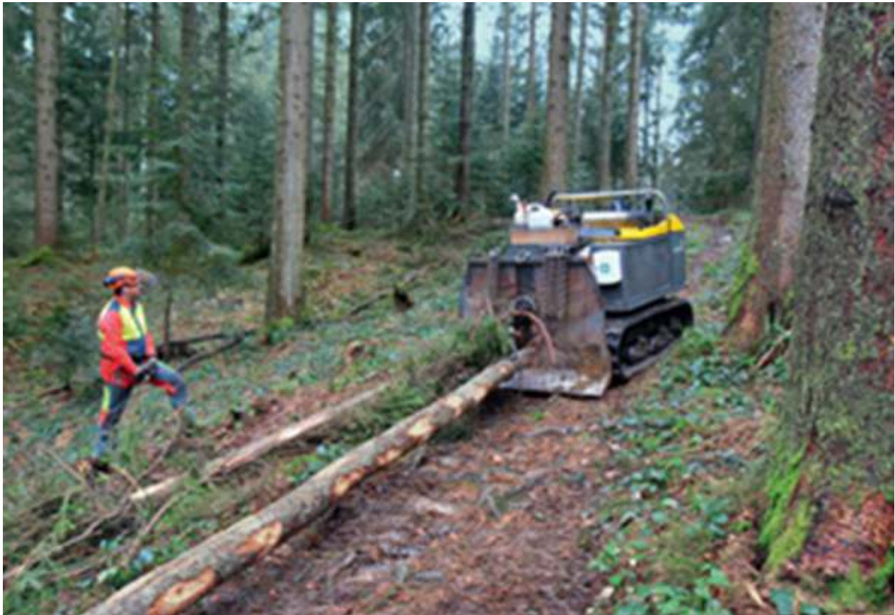
Figure 7. Alther Raup track rubber tracked forwarding winch ( www.martin-alther.ch ).
