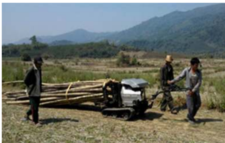
Figure 16. Forwarding delimited bamboo culms by local mini-skidder
