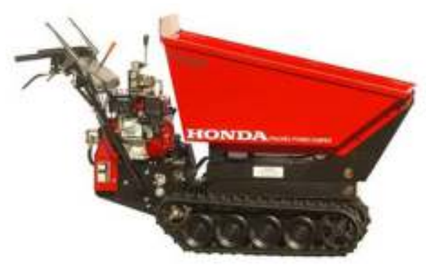
Figure 11. Honda TD 500 (650) mini-dumper
