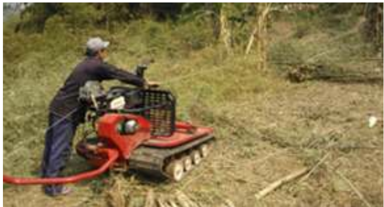
Figure 13. Iron Horse power winch used to extract bundles of entangled bamboo.
