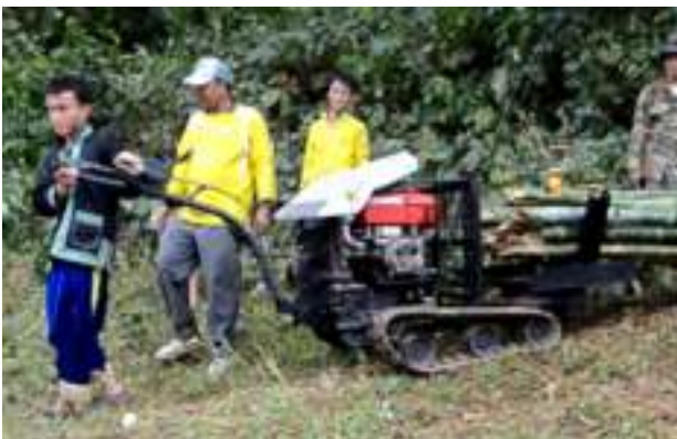
Figure 12. Yanmar bamboo crawler with engine in reverse position and clamping device for bamboo poles
