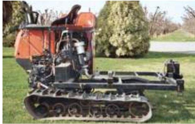
Figure 9. Kubota Rice harvester (3 cylinder diesel 18 hp) rubber-tracked base ( www.plunkettorchards.com.au ).
