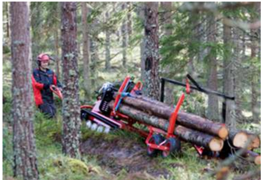
Figure 1. A 9 hp Iron Horse with hydraulic winch, sidewise loading boom and log trailer.
