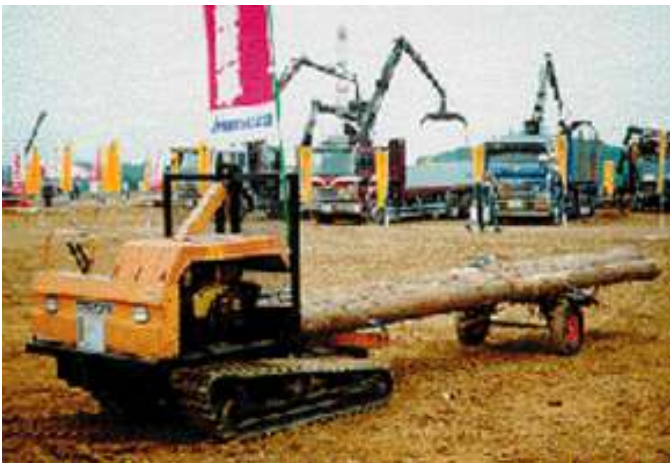
Figure 6. Hitachi CG 8 7hp 800 kg load capacity Irish R pound 9500
