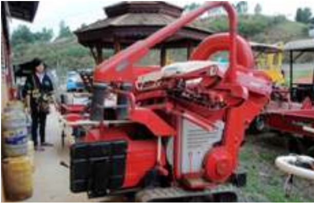
Figure 8. The Yanmar 9HP rice thresher before conversion, note the white handle for forward movement of the machine
