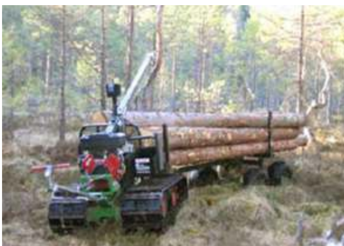
Figure 3. The Myreback Gustafsson-Oxen mini skidder with loading boom and log trailer www.myreback.com
